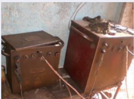
Transformer oil-based welding machines
