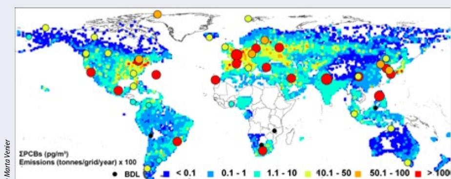
Mean concentrations (pg.m<sup>-3</sup>) in air for PCBs during 2005 superimposed on 2005 PCB inventory by Brevik et al. 2007. From Pozo et al. (2009)
