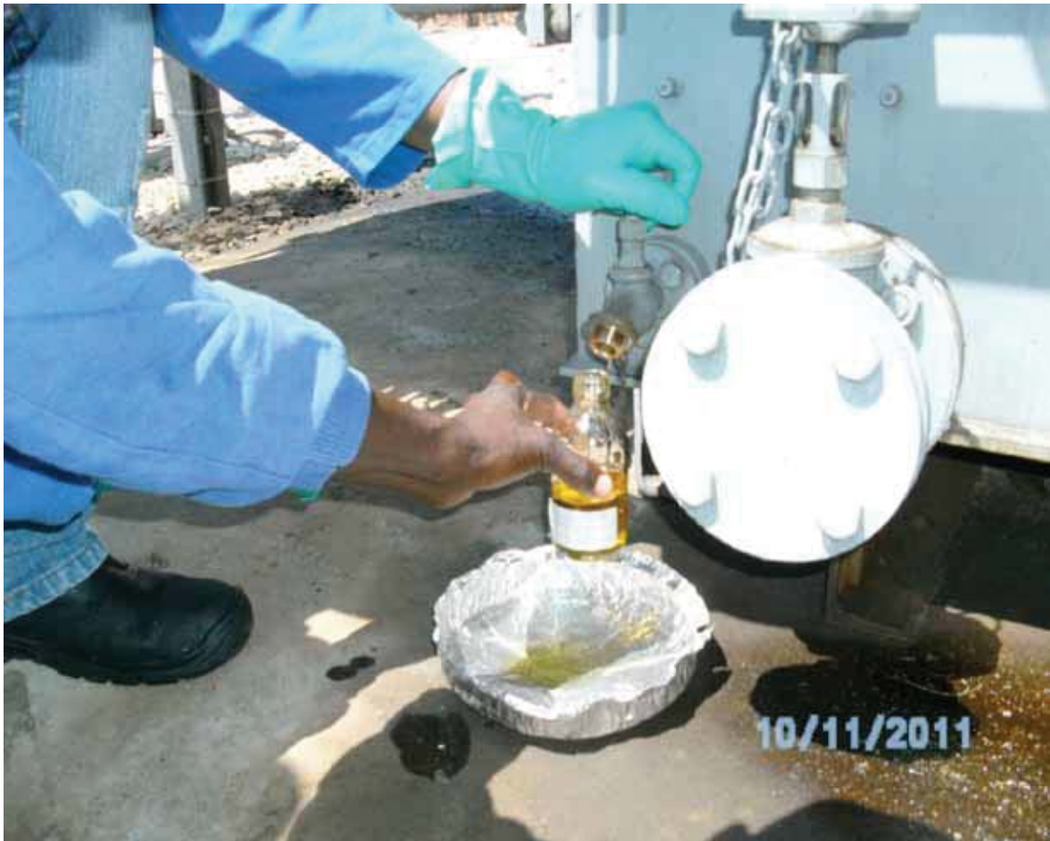
Figure 8 showing a seasoned worker handling transformer oil with bare hands (Source: MENRM, 2012 PCB Inventory Report for Zimbabwe 2011)
