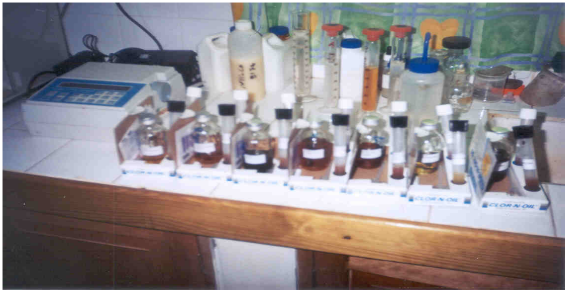
Figure 2.3.2.3: Samples of transformer oil and results obtained with the PCB test kits at the laboratory of the Ministry of Environment, in December 2004
