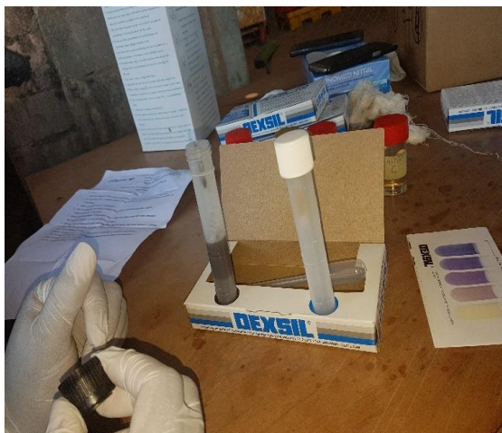
Figure 3.4: Workers of the Cahora Bassa Dam during the qualitative analysis of the chlorine content by the CLOR_ON_OIL method in 2018.
