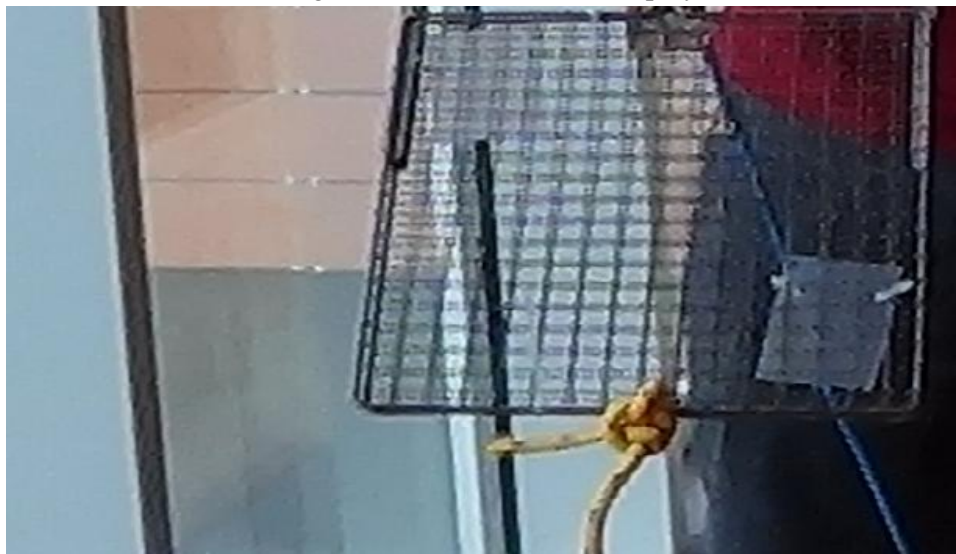
Figure 17: Photo showing sampler employing Semi-Permeable Membrane Devices
