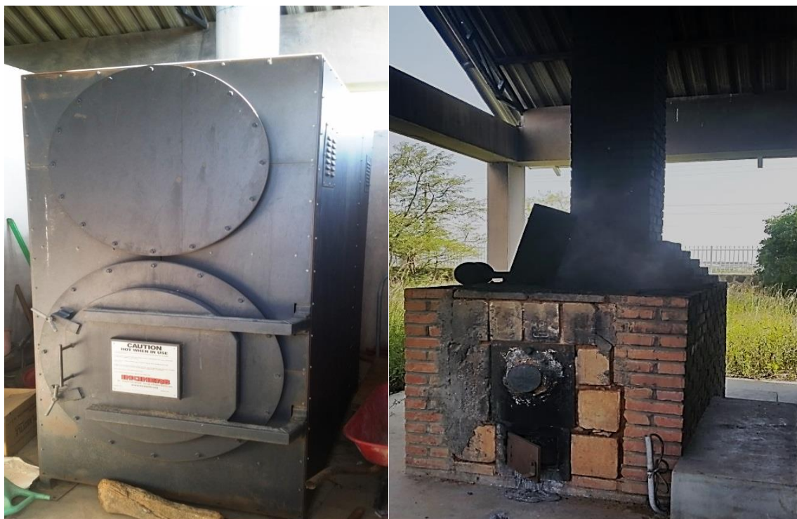
Figure 16: Electrical (left) and manual (right) incinerator facilities
