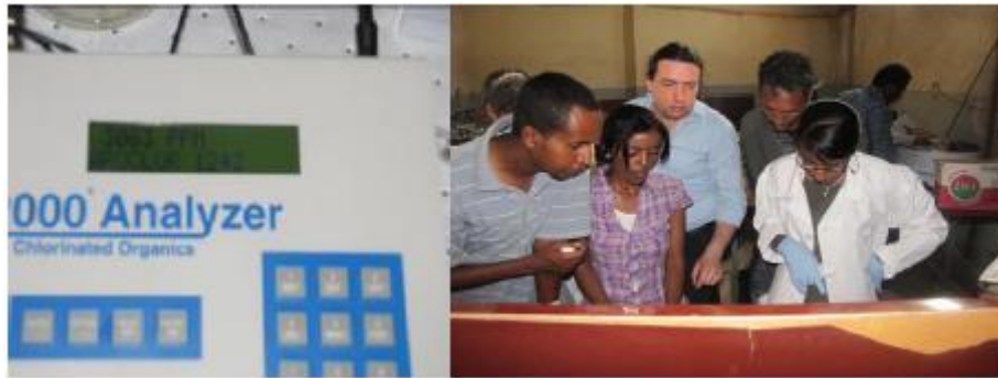
Screening of PCB via L-2000 analyzer in water resources laboratory
