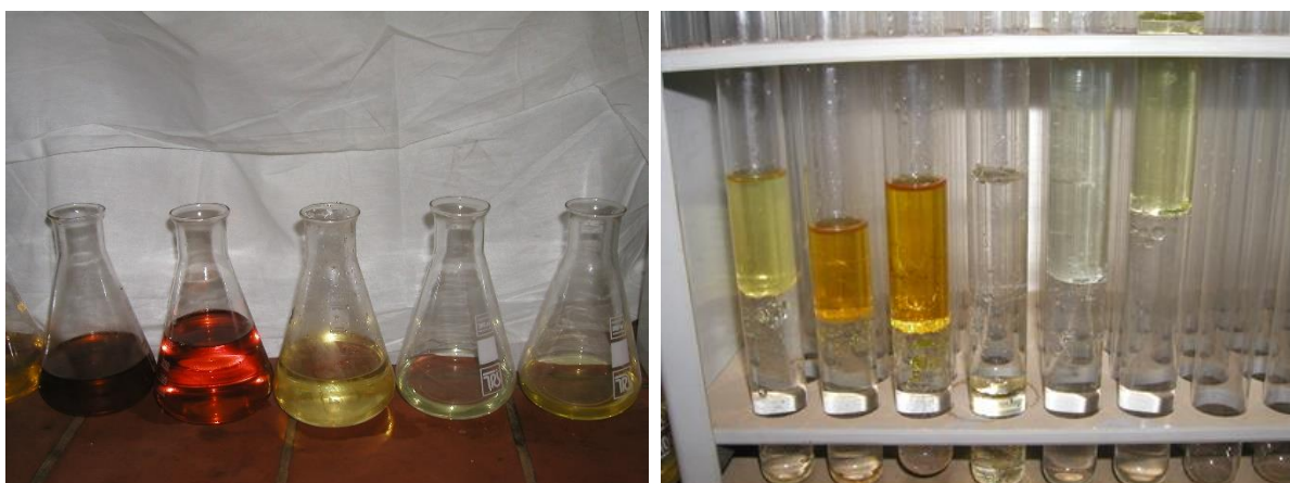
Figure 5: Density test: transformer oils sampled (left); transformer oils with water in test tubes (right)
