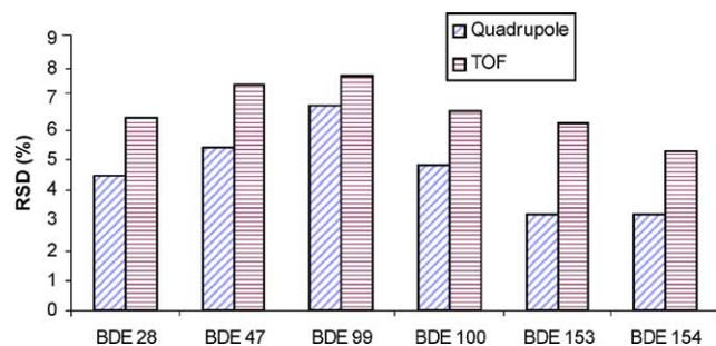
Fig. 2. Comparison of intra-day repeatability of GC-TOF-MS and GC-MS quadrupole analysis.
