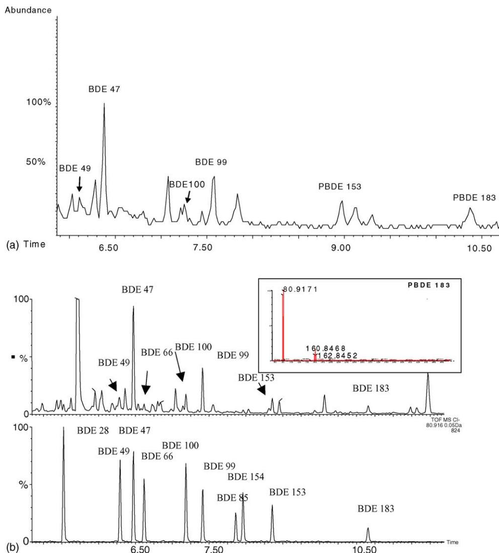
Fig. 1. (a) Chromatogram of milk sample (M 61) analysed by GC-MS with quadrupole analyzer operated in the NCI mode (injection equivalent to 1.2 mg of lipids); (b) chromatogram of milk sample (M 61) analysed by GC-MS with TOF analyzer operated in the NCI mode (injection equivalent to 0.6 mg of lipids) with NCI spectrum of BDE 183, time scale in minutes.
