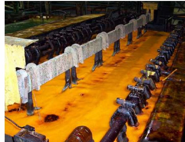
Hard Chrome Bath with Fumetrol® 21 (non-PFOS mild foaming mist suppressant)
