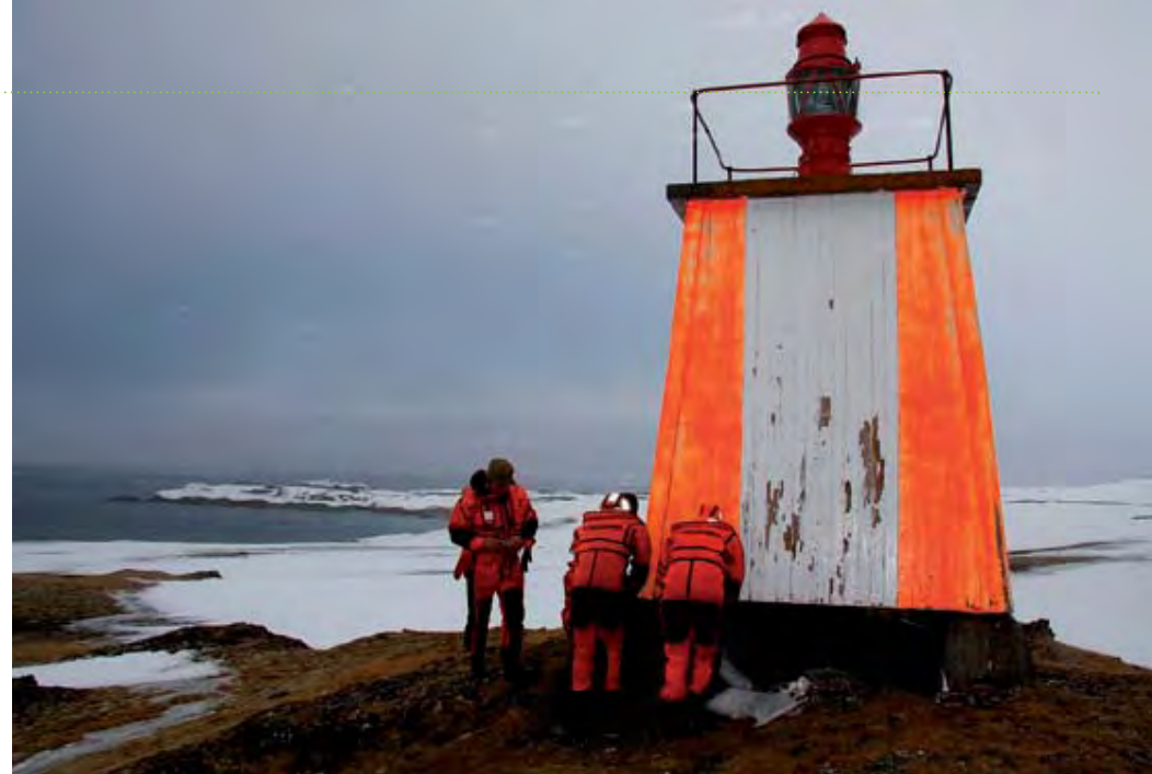
Paint samples collected from lighthouse Fuglehuken. Picture taken by Halvard Pedersen at the Governor of Svalbard
