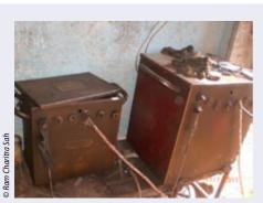
Transformer oil-based welding machines
