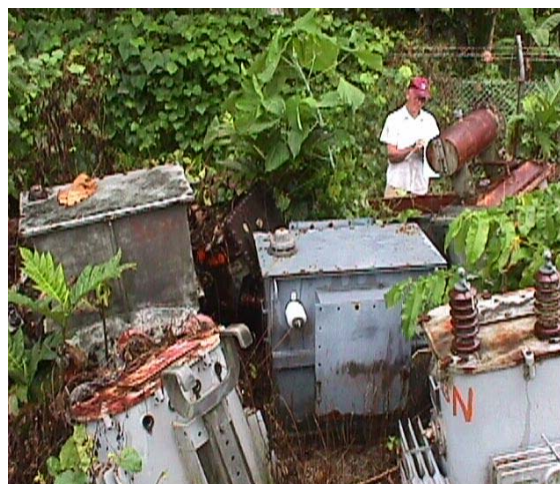
Figures 9 (left): Copper-chrome-arsenic contamination at the SFP, Asau Figure 10 (right): Transformers including PCB -contaminated at EPC depot, Vaitele
