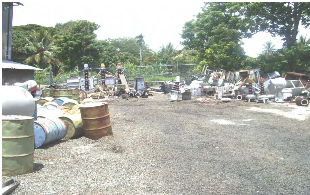
Figure 5: Obsolete Stockpile of Equipment that could contain PCBs and produce dielectric fluids
