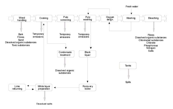
Figure 5 Emissions to air, kraft pulp mill example - [EIPPCB BREF, 2001]
