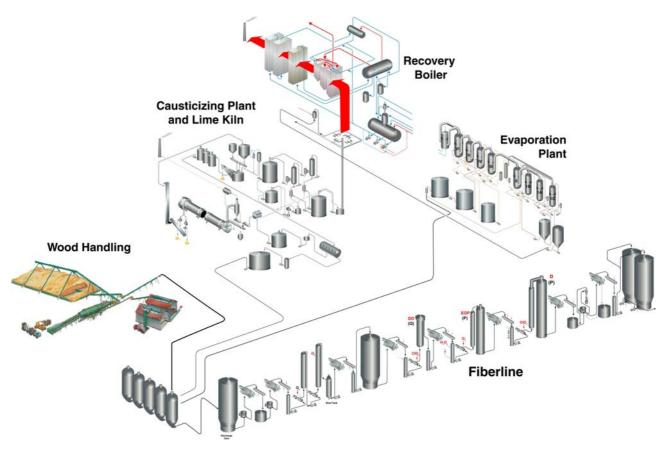
Figure 1. Example of a modern ECF kraft wood pulping mill - Courtesy of Metso Automation Inc. 2003
