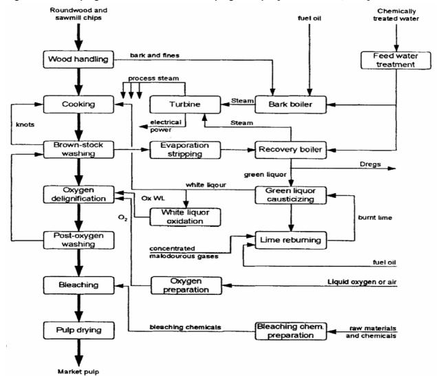
Figure 2. Pulping Process Flows – Kraft Pulping Example [EIPPCB BREF, 2001]
